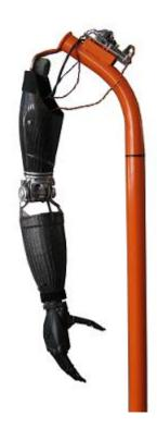
images with a single camera, work out how to modify a prosthetic arm to enable computer control, design wearable markers which could be tracked by the camera and create a computer program to track the markers. This tracking information was then used to program the prosthetic arm to allow it to perform the desired actions.
